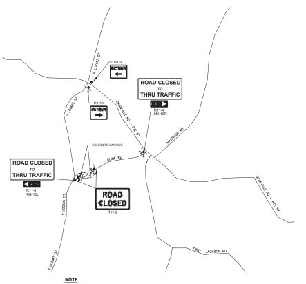
COORDINATE FINAL LOCATIONS OF TEMPORARY TRAFFIC CONTROL DEVICES WITH THE ENGINEER PRIOR TO PLACEMENT
